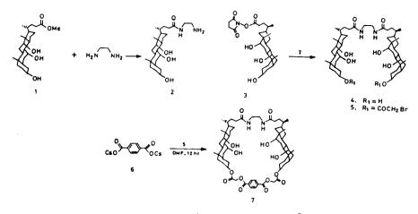
the products were characterized by IR and <sup>1</sup>H-NMR spectroscopy<sup>7</sup>. No higher oligomer was detected in HPLC.
